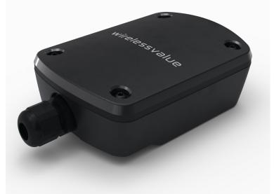
The Wireless Value DLXa measures process signals and transmits data to the base station. Sensing is performed using any available sensor with 0- 25 mA output. This allows connection of numerous commercially available sensors to monitor a wide variety of measurement parameters such as flow, level, pressure etc.
