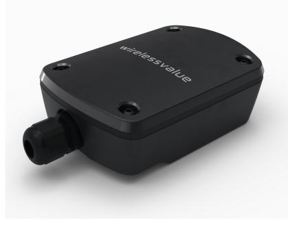
The Wireless Value DLXm measures process signals and transmits data to the base station. Sensing is performed using any available sensor with 0 – 1 V DC output. This allows connection of numerous commercially available sensors to monitor a wide variety of measurement parameters such as flow, level, pressure etc. With the reference output of 2.45 V this sensor is also suitable for Strain Gauge measurement (load cells etc.).
