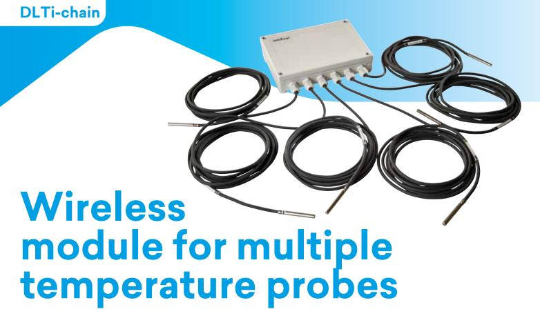
The Wireless Value DLTi-chain measures 2 to 6 temperatures and transmits data to the base station. Sensing is performed using extended watertight probes. The probes are available in two standard lengths - 2 meters and 5 metres. The probes are digital temperature probes with the same form factor as a PT1000.
